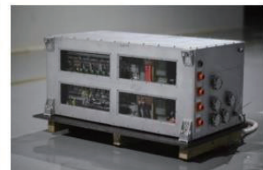
Hydrogen power generation module unit (reactor module) 1150*660*476mm
